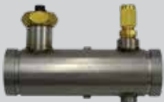
Manifold Prevents backflow to fire pump. Stainless steel, brass components and construction. Includes flow sensor mount, water way check valve, check valve injector port, and a drain. Available in 1.5", 2.0", 2.5", 3", and 4" victaulic.
