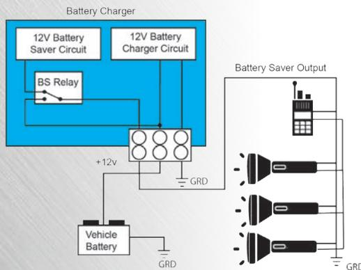
**Battery Saver Operation:** When the battery charger is operating, the vehicle's accessories are powered by the 12V battery saver circuit, internal to the charger. When the charger is powered off, a relay inside the charger switches the vehicle accessories directly to the battery.
