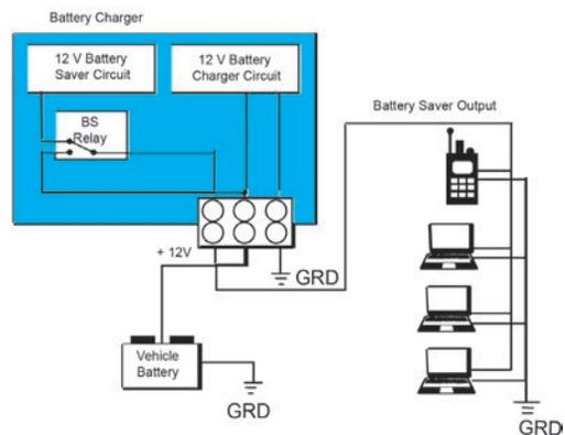
**Battery Saver Operation:** When the battery charger is operating, the vehicle's accessories are powered by the 12V battery saver circuit, internal to the charger. When the charger is powered off, a relay inside the charger switches the vehicle accessories directly to the battery.
