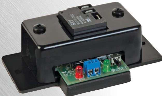
The 091-108-012 Over Voltage Relay continuously monitors the voltage of the battery. The unit is factory set to actuate at 17V, reset at 14V, and may be adjusted to other voltage trigger points. The output relay is capable of switching 30A, and both "Normally Open" and "Normally Closed" contacts are provided.
